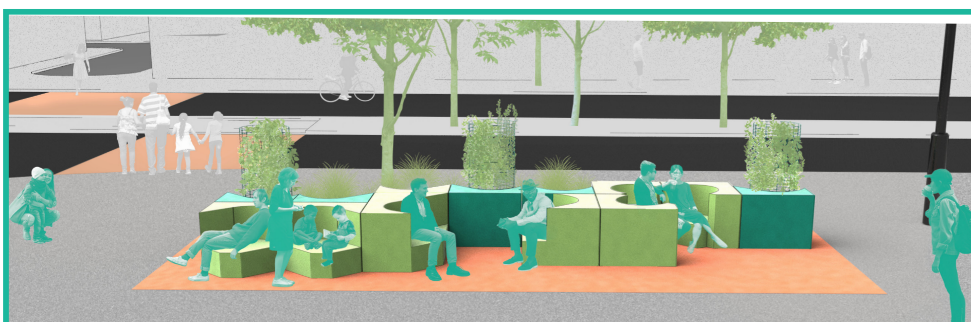
10 Modular components generate a greening strategy for the area, with planting and seating that can be used to create a visual and acoustic barrier from the road, soften the pavement, and offer a more pleasant atmosphere for the pedestrian. Some of these elements incorporate bike/scooter parking as well as bins to keep the area tidy.
